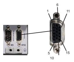
Figure 7. Feedback Connection
