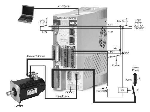
Figure 1. Minimum Wiring for Drive Operation
