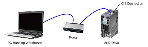
Figure 14. Option B: Connection to a Router
