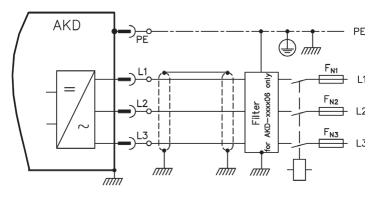
Figure 10. AC Input Power Wiring Diagram
