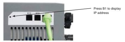
Figure 16. IP Address Display Button B1
