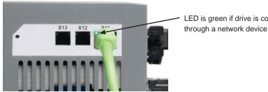
Figure 15. Active connection LED
