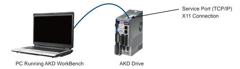
Figure 12. Option A: Direct Connection
