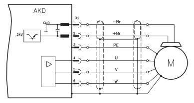
Figure 6. Motor Power Wiring Details, Cable length <= 25 m
